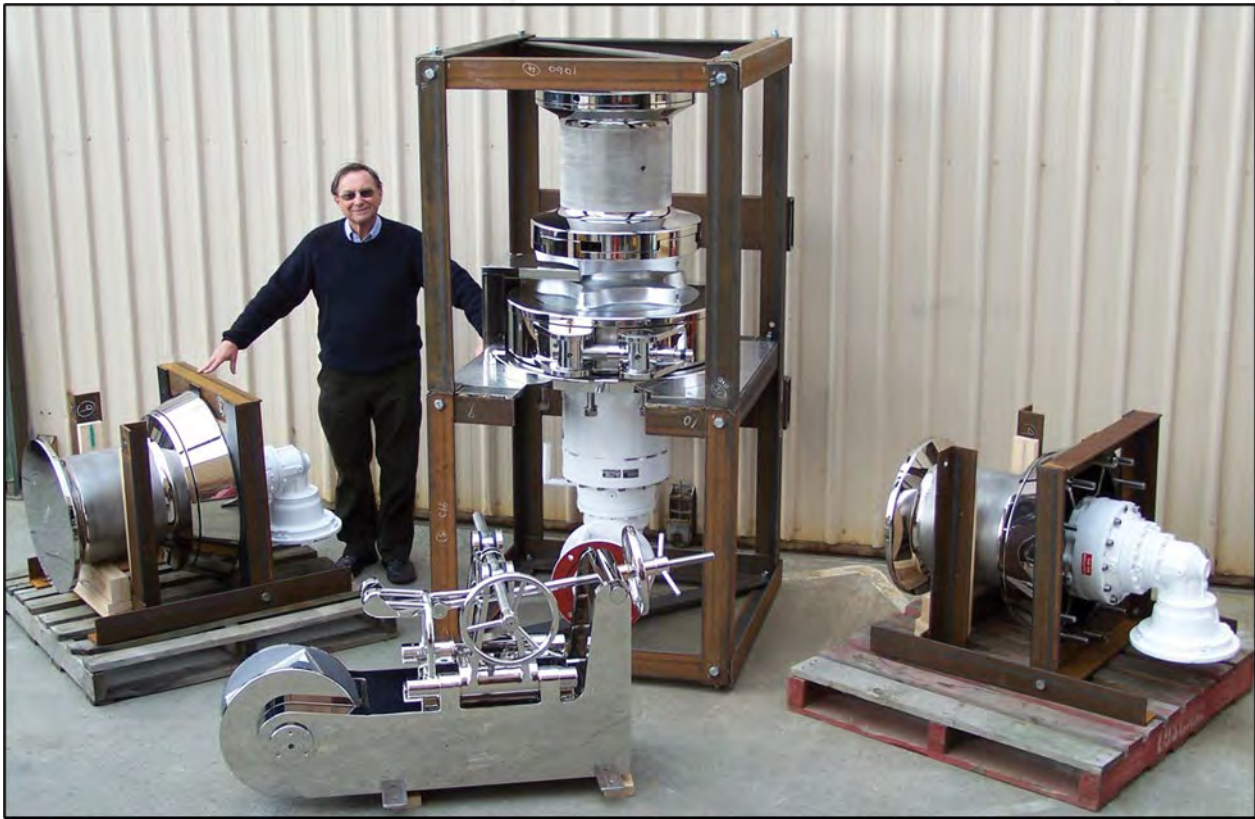
2009: John with Muir's largest winch at the time, the VRC 24000. Muir can now construct up to a VRC 40000.
