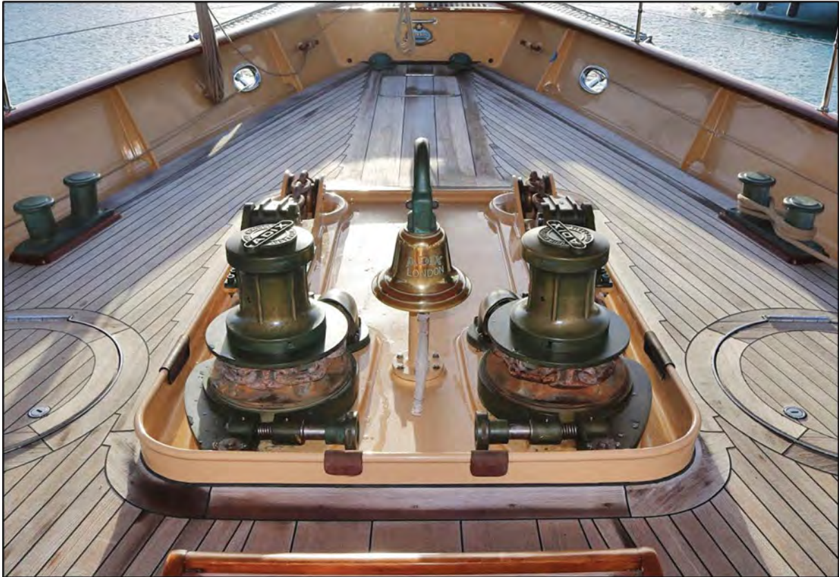
1997 (Photo in 2016): Sailing Yacht Adix's Aluminium Bronze Windlasses
