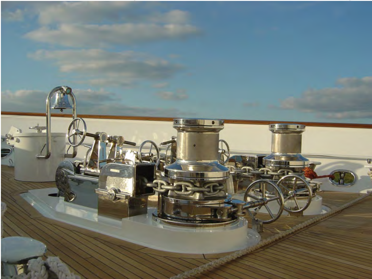
2005: VRC 20000s and Chain Compressors on board Feadship Rasselas
