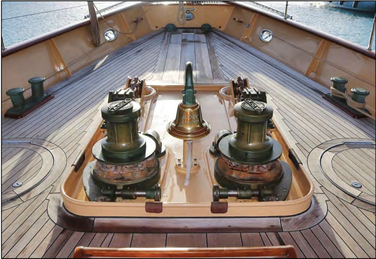
1997(Photo in 2016): Sailing Yacht Adix's Aluminum Bronze Windlasses.
